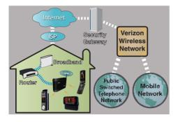
About the size of a traditional wireless access point (WAP), the base station facilitates the delivery of cellular traffic through the Internet to the Verizon Wireless network, which then routes the signal to the desired party.
